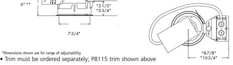
GUIDELINES MIN MAX REQUIRES SD HOUSING OPTION 7-15/16 8-1/8 ALL STANDARD HOUSINGS 8-1/8 8-3/4 REQUIRES P8101-01 KIT 8-3/4 9-1/8 ACCESSORY & WF REFLECTOR
