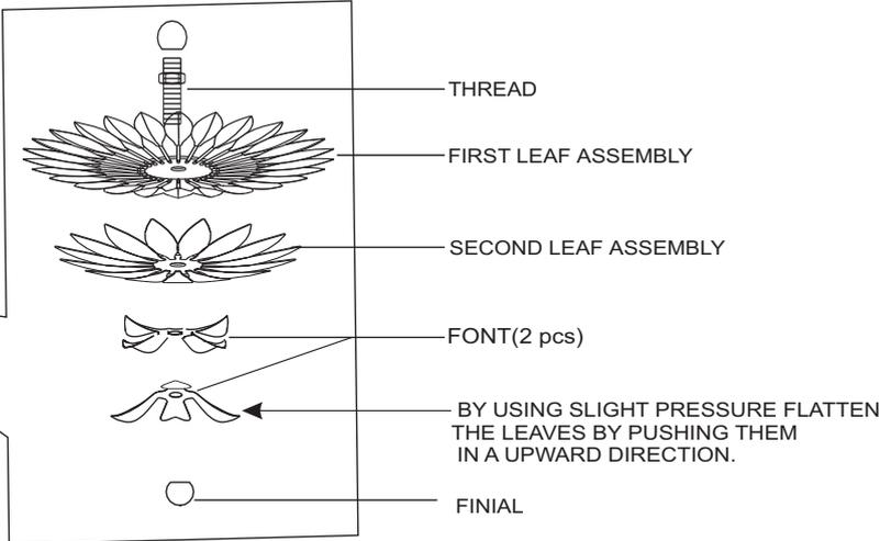
ASSEMBLE THESE PARTS TO THE BOTTOM
